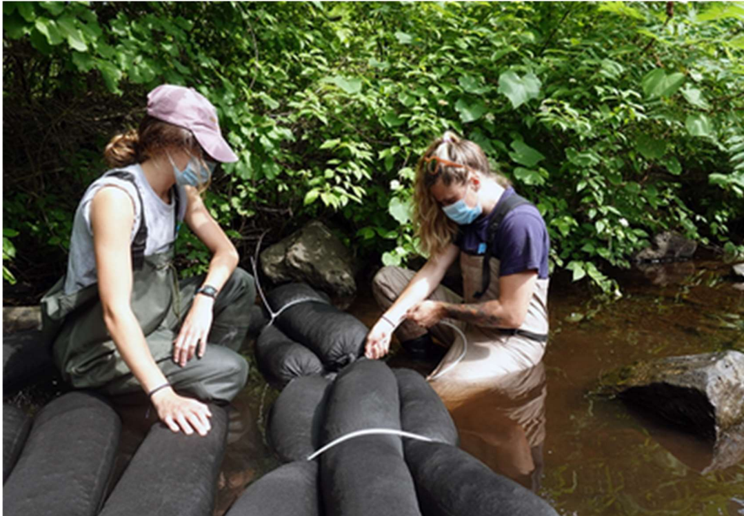
Figure VI-5. Biochar socks installed in Lake Hopatcong, NJ. The New Jersey Department of Environmental Protection recently provided a grant to the Lake Hopatcong Commission to test biochar use in an effort to adsorb phosphorus from lake water. Lake Hopatcong is a 14 m deep, ~2,600 acre lake/reservoir with a phosphorus TMDL and a lake management organization, the Lake Hopatcong Commission. Source: https://www.lakehopatcongfoundation.org/news/biochar-installations (accessed 9/5/22).
