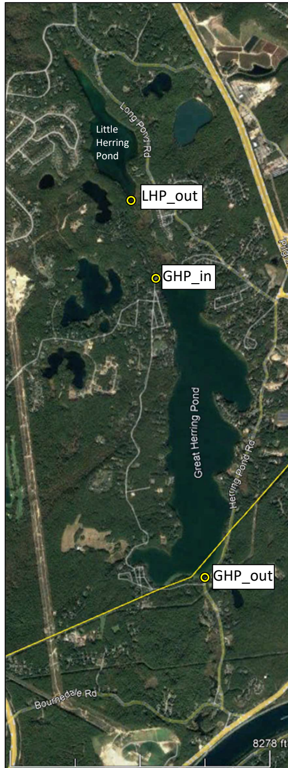
Figure IV-7. GHP and LHP Streamflow Monitoring Locations. HPWA measured streamflow at the outlet from Little Herring Pond (LHP_out), the inlet to Great Herring Pond (GHP_in) and the outlet from Great Herring Pond (GHP_out). CSP/SMASST collected measurements at LHP_out and GHP_out during 2021.
