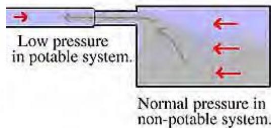
Outside water taps and garden hoses tend to be the most common sources of cross connection contamination at home. The garden hose creates a hazard when submerged in a swimming pool or when attached to a chemical sprayer for weed control. Garden hoses that are left lying on the ground may be contaminated by fertilizers, cesspools, or garden chemicals.
