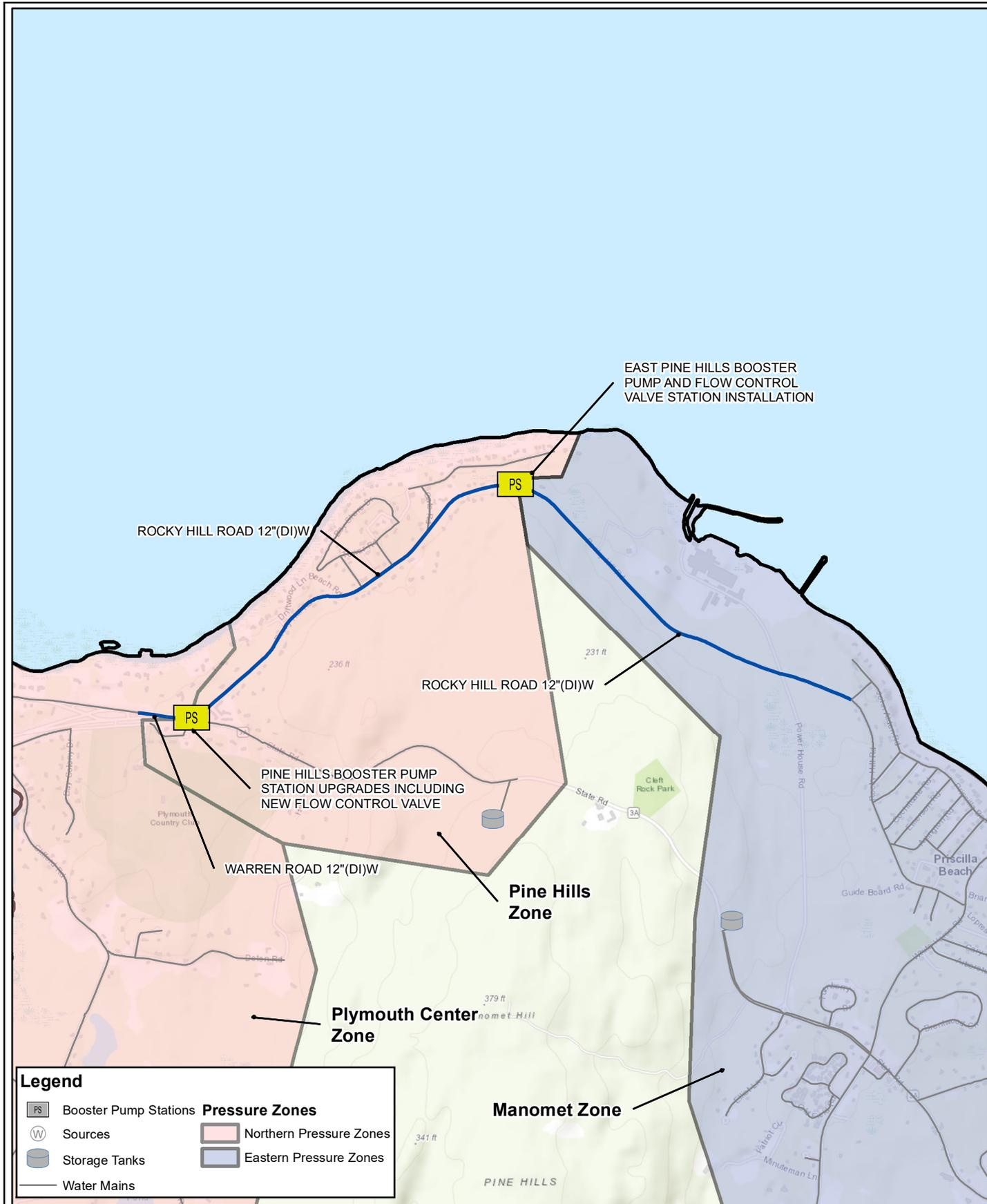
EAST PINE HILLS BOOSTER PUMP AND FLOW CONTROL VALVE STATION INSTALLATION
