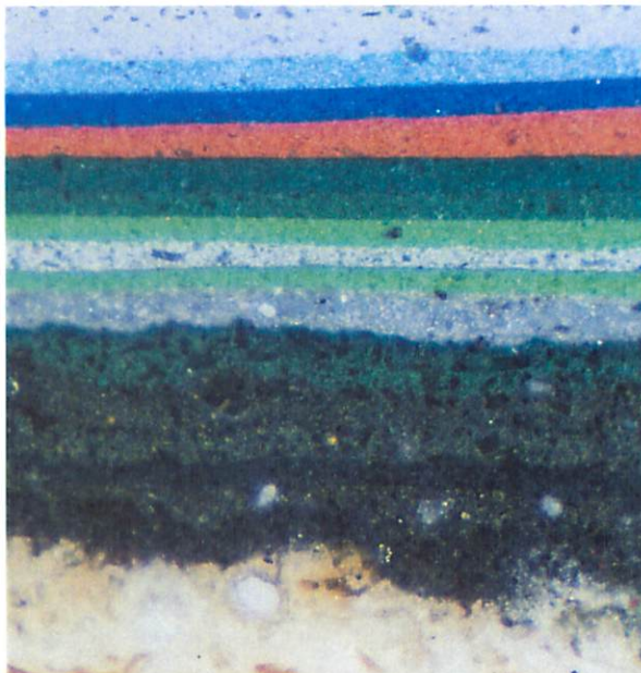
Microscope photo 8 - Cross section at 100x of sample from beaded boards forming the panels of the entry doors. The off-white at the bottom is a primer. The first five or six generations are all dark greens. Although very dark, they appear to be greener than the dark blackish green on the trim.
