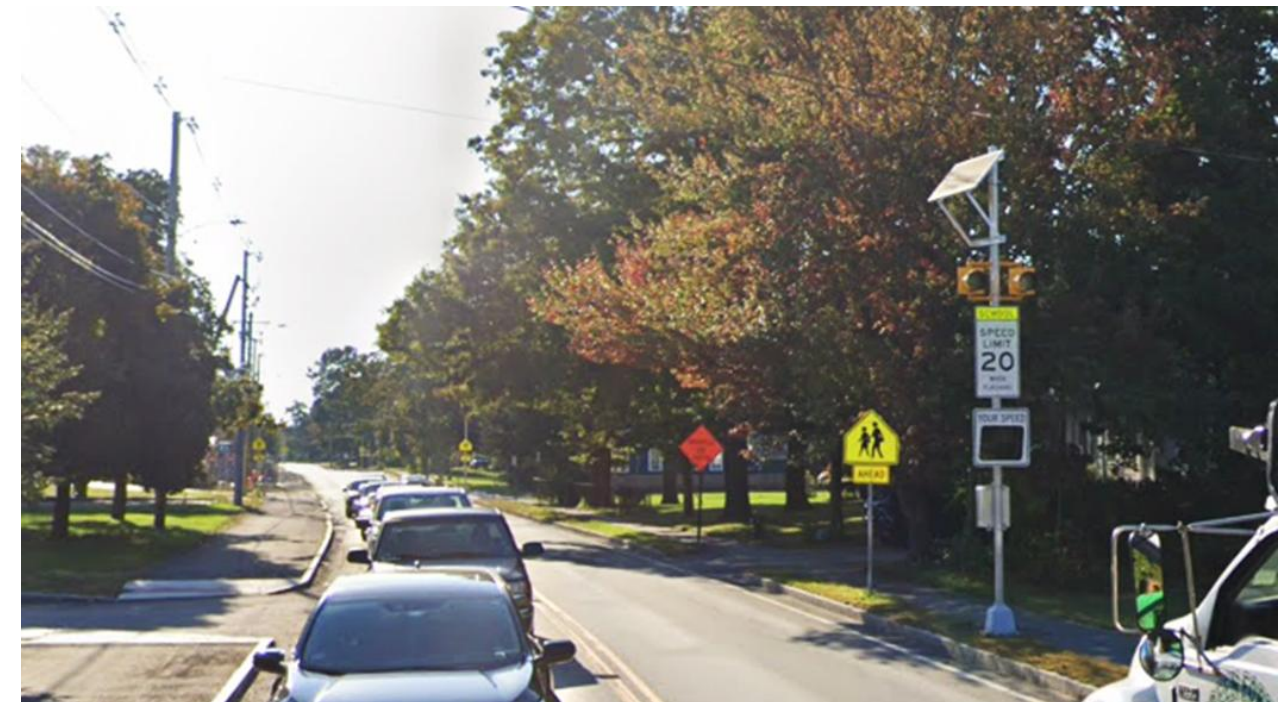
Figure 17. Example Enhanced School Zone Speed Sign with Dynamic Speed Feedback Sign
