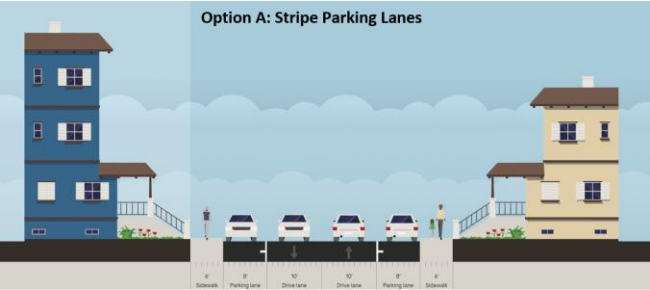
Figure 46. Option A Option A would stripe the roadway to two 10’ travel lanes and 8’ parking lanes. While this may deter residents from parking on sidewalks, in areas where parking is sparse, this still results in a wide expanse of pavement and therefore speeding may persist.
