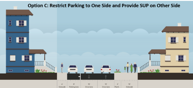
Figure 48. Option C Option C would restrict parking to one side of the roadway and provide a SUP on the other side to accommodate the school traffic along the corridor. This would deter vehicles from parking on sidewalks as well as reduce the curb-to-curb width- reducing vehicle speeds along the corridor.
