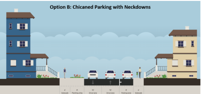
Figure 47. Option B Option B would chicane the parking along the corridor (i.e., periodically switching the side parking is located on and providing physical neckdowns on the other side to horizontally deflect travel and reduce speeds). In some scenarios, this may cause residents to park on the other side of their residence and have to cross the street. Therefore, parking locations should be thoughtfully considered regarding current parking patterns and ensure that crossings are enhanced along the corridor. In areas with neckdowns, the curb-to-curb width would narrow, reducing speeds along the corridor
